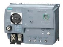
SIRIUS motor starter M200D AS-i Communication: AS-Interface DOL starter Basic Mechanical switching AC-3, 5.5 kW / 400 V 1.5 A...12.00 A Electronic overload protection Thermistor: THERMOCLICK / PTC with brake contact 400 V AC 2DI AS-i + 2DI / 1DO on device Han Q4/2 - Han Q8/0 with manual on-site operation and key-operated switch
