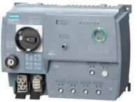
SIRIUS motor starter M200D AS-i Communication: AS-Interface Reversing starter Basic Electronic switching AC-3, 0.75KW / 400 V 0.15 A...2.00 A Electronic overload protection Thermistor: THERMOCLICK / PTC without brake contact 2DI AS-i + 2DI / 1DO on device Han Q4/2 - Han Q8/0 with manual on-site operation and key-operated switch
