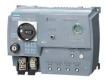
SIRIUS motor starter M200D AS-i Communication: AS-Interface DOL starter Basic Electronic switching AC-3, 0.75KW / 400 V 0.15 A...2.00 A Electronic overload protection Thermistor: THERMOCLICK / PTC with brake contact 180 V DC 2DI AS-i + 2DI / 1DO on device Han Q4/2 - Han Q8/0 with manual on-site operation and key-operated switch
