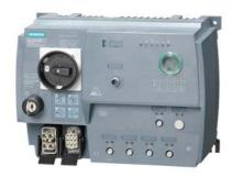
SIRIUS motor starter M200D AS-i Communication: AS-Interface DOL starter Basic Electronic switching AC-3, 0.75KW / 400 V 0.15 A...2.00 A Electronic overload protection Thermistor: THERMOCLICK / PTC without brake contact 2DI AS-i + 2DI / 1DO on device Han Q4/2 - Han Q8/0 with manual on-site operation and keyoperated switch
