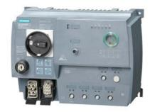
SIRIUS motor starter M200D AS-i Communication: AS-Interface Reversing starter Basic Mechanical switching AC-3, 0.75KW / 400 V 0.15 A...2.00 A Electronic overload protection Thermistor: THERMOCLICK / PTC with brake contact 180 V DC 2DI AS-i + 2DI / 1DO on device Han Q4/2 - Han Q8/0 with manual on-site operation and key-operated switch
