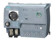
SIRIUS motor starter M200D AS-i Communication: AS-Interface DOL starter Basic Mechanical switching AC-3, 0.75KW / 400 V 0.15 A...2.00 A Electronic overload protection Thermistor: THERMOCLICK / PTC with brake contact 180 V DC 2DI AS-i + 2DI / 1DO on device Han Q4/2 - Han Q8/0 with manual on-site operation and key-operated switch
