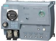
SIRIUS motor starter M200D AS-i Communication: AS-Interface DOL starter Basic Mechanical switching AC-3, 0.75KW / 400 V 0.15 A...2.00 A Electronic overload protection Thermistor: THERMOCLICK / PTC with brake contact 400 V AC 2DI AS-i + 2DI / 1DO on device Han Q4/2 - Han Q8/0 with manual on-site operation and key-operated switch
