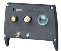
SIRIUS motor starter M200D communication module PROFIBUS DP removable Bus connection 2 x M12 with loop-through Power connection 24 V 2 x 7/8" with loop-through Bus terminating resistor integrated via technology module 3RK1395\* can be used as Motor starter M200D with communication
