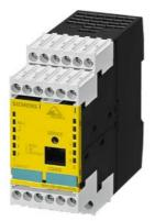
ASIsafe Basis Safety monitor 2 F-RO 2 enabling circuits IP20, with screw terminal removable terminals Safe output relay Response time maximum 40 ms Monitor type 2, Version 3 Can be used up to Category 4 (EN954-1) up to PL E (EN ISO 13849-1) up to SIL 3 (IEC 61508)
