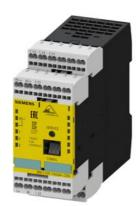
ASIsafe extended Safety monitor 1 F-RO 1 enabling circuit IP20, with spring-type terminal removable terminals Safe output relay Response time maximum 40 ms Monitor type 3, Version 3 Can be used up to Category 4 (EN954-1) up to PL E (EN ISO 13849-1) up to SIL 3 (IEC 61508)
