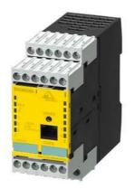
ASIsafe extended Safety monitor 1 F-RO 1 enabling circuit IP20, with screw terminal removable terminals Safe output relay Response time maximum 40 ms Monitor type 3, Version 3 Can be used up to Category 4 (EN954-1) up to PL E (EN ISO 13849-1) up to SIL 3 (IEC 61508)
