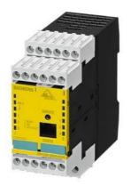
ASIsafe Basis Safety monitor 1 F-RO 1 enabling circuit IP20, with screw terminal removable terminals Safe output relay Response time maximum 40 ms Monitor type 1, Version 3 Can be used up to Category 4 (EN954-1) up to PL E (EN ISO 13849-1) up to SIL 3 (IEC 61508)
