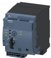
SIRIUS Compact load feeder Reversing starter for IO-Link 690 V 24 V DC 0.32...1.25 A IP20 Connection main circuit: plug-in, without terminals Connection control circuit: Spring-type terminal
