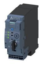
SIRIUS Compact load feeder DOL starter for IO-Link 690 V 24 V DC 1...4 A IP20 Connection main circuit: plug-in, without terminals Connection control circuit: Spring-type terminal
