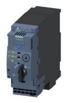
SIRIUS Compact load feeder DOL starter for IO-Link 690 V 24 V DC 0.32...1.25 A IP20 Connection main circuit: plug-in, without terminals Connection control circuit: Spring-type terminal
