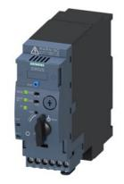
SIRIUS Compact load feeder DOL starter for IO-Link 690 V 24 V DC 8...32 A IP20 Connection main circuit: plug-in, without terminals Connection control circuit: screw terminal
