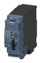
SIRIUS Compact load feeder DOL starter for IO-Link 690 V 24 V DC 3...12 A IP20 Connection main circuit: plug-in, without terminals Connection control circuit: screw terminal
