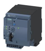
SIRIUS Compact load feeder Reversing starter 690 V 110...240 V AC/DC 50...60 Hz 3...12 A IP20 Connection main circuit: plug-in, without terminals Connection control circuit: Spring-type terminal
