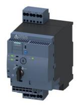
SIRIUS Compact load feeder Reversing starter 690 V 24 V AC/DC 50...60 Hz 3...12 A IP20 Connection main circuit: Spring-type terminal Connection control circuit: Spring-type terminal
