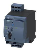
SIRIUS Compact load feeder Reversing starter 690 V 24 V AC/DC 50...60 Hz 0.1...0.4 A IP20 Connection main circuit: Spring-type terminal Connection control circuit: Spring-type terminal
