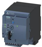
SIRIUS Compact load feeder Reversing starter 400 V 24 V AC/DC 50...60 Hz 8...32 A IP20 Connection main circuit: plug-in, without terminals Connection control circuit: screw terminal
