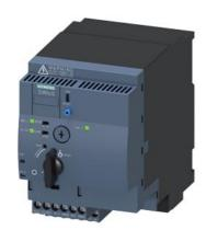
SIRIUS Compact load feeder Reversing starter 690 V 24 V AC/DC 50...60 Hz 0.32...1.25 A IP20 Connection main circuit: plug-in, without terminals Connection control circuit: screw terminal
