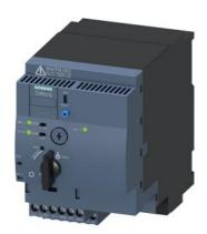
SIRIUS Compact load feeder Reversing starter 690 V 110...240 V AC/DC 50...60 Hz 0.1...0.4 A IP20 Connection main circuit: plug-in, without terminals Connection control circuit: screw terminal
