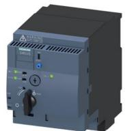
SIRIUS Compact load feeder Reversing starter 690 V 24 V AC/DC 50...60 Hz 3...12 A IP20 Connection main circuit: plug-in, without terminals Connection control circuit: plug-in, without terminals
