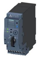
SIRIUS Compact load feeder DOL starter 690 V 110...240 V AC/DC 50...60 Hz 8...32 A IP20 Connection main circuit: plug-in, without terminals Connection auxiliary circuit: screw terminal
