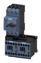
Load feeder fuseless, Reversing duty 400 V AC, Size S00 0.28...0.40 A 230 V AC screw terminal for installation on standard mounting rail (also fulfills type of coordination 1) Type of coordination 2, Iq = 150 kA 1 NC (contactor)
